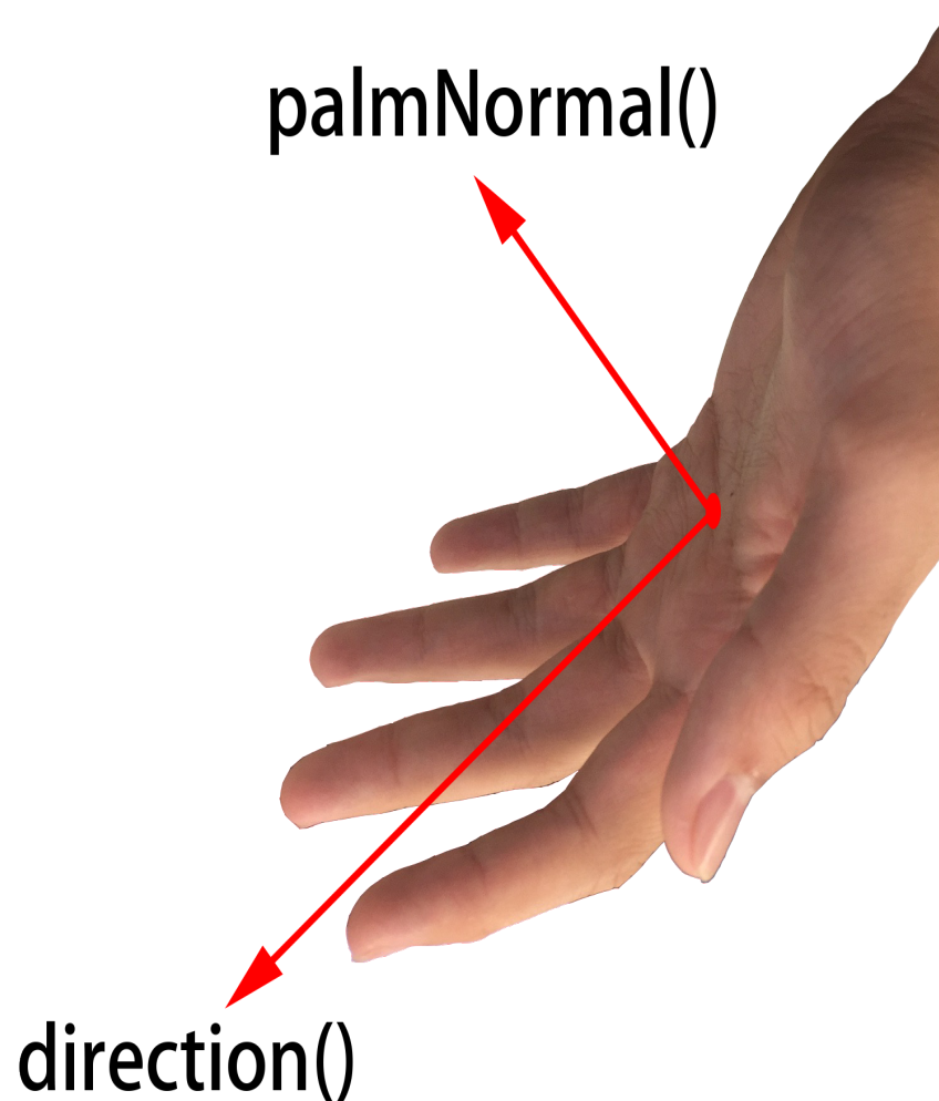
Figure 3.2 The Hand palmNormal() and direction() vectors define the orientation of the hand.
