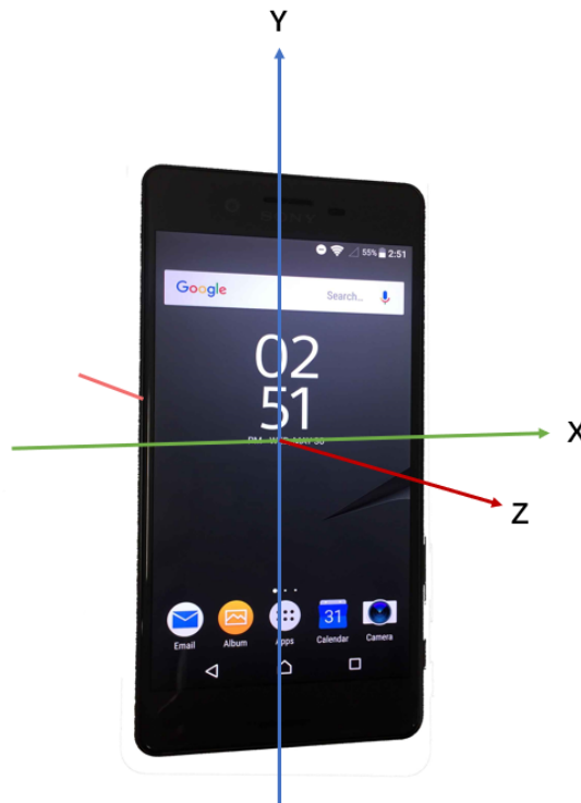
Figure 5.3 Android smartphone and the coordinate system used by the sensor framework
