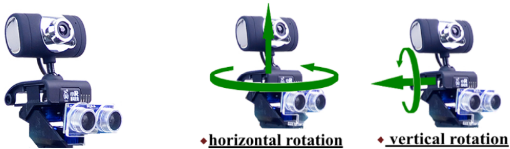
Fig. 3.5 The two-direction rotation of pan-tilt
