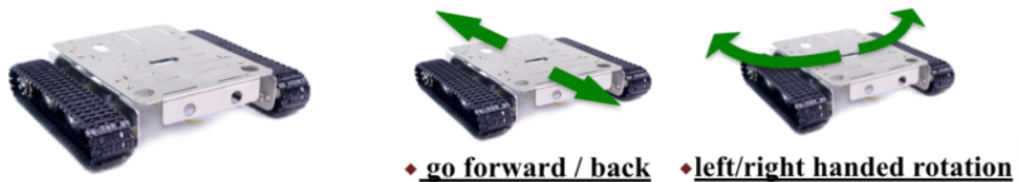
Fig. 3.6 The translation and rotation of caterpillar band
