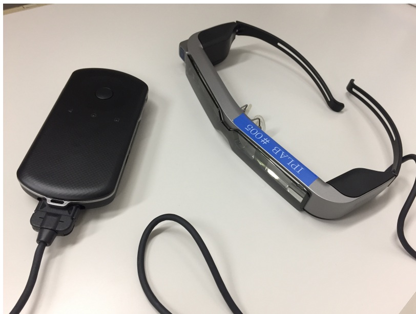
Fig. 2.2 HMD: Epson moverio bt-300
