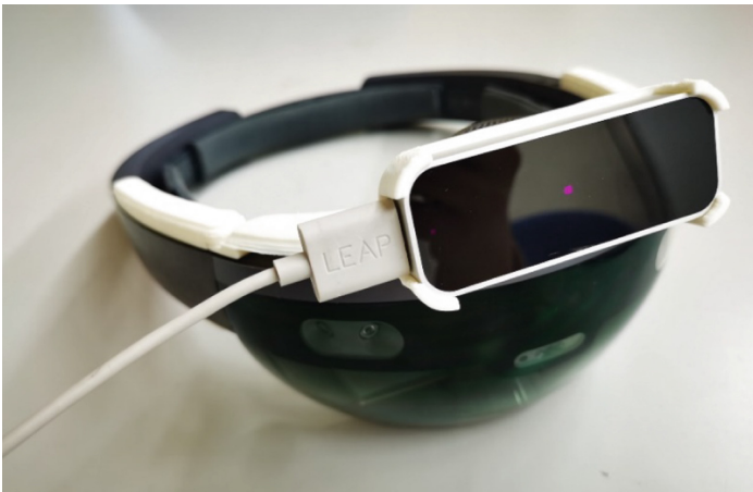
Fig. 9. Device assembly for attaching Leap Motion to HoloLens 1.
