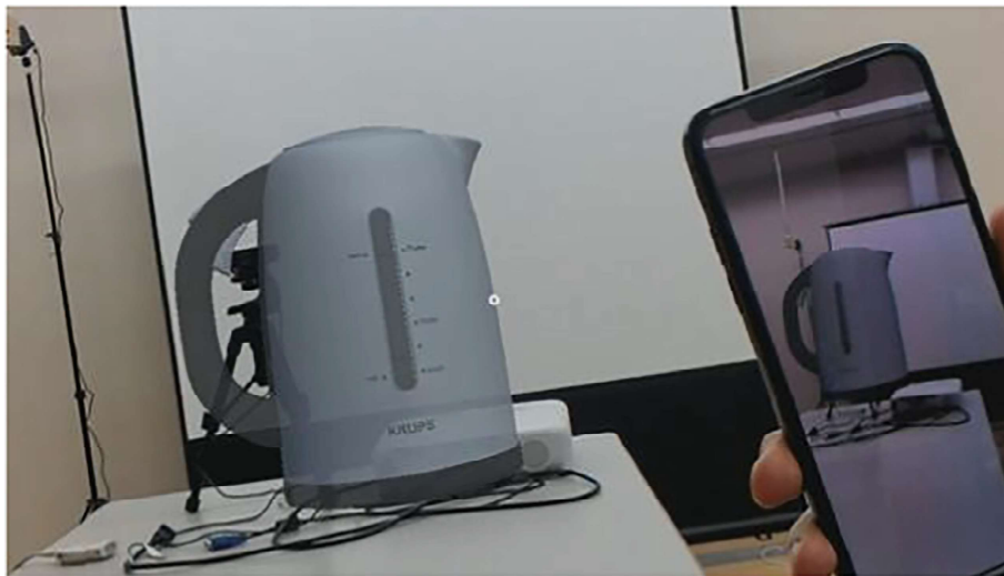
Fig. 8. Synchronized virtual object showed in smartphone (captured by HMD)
