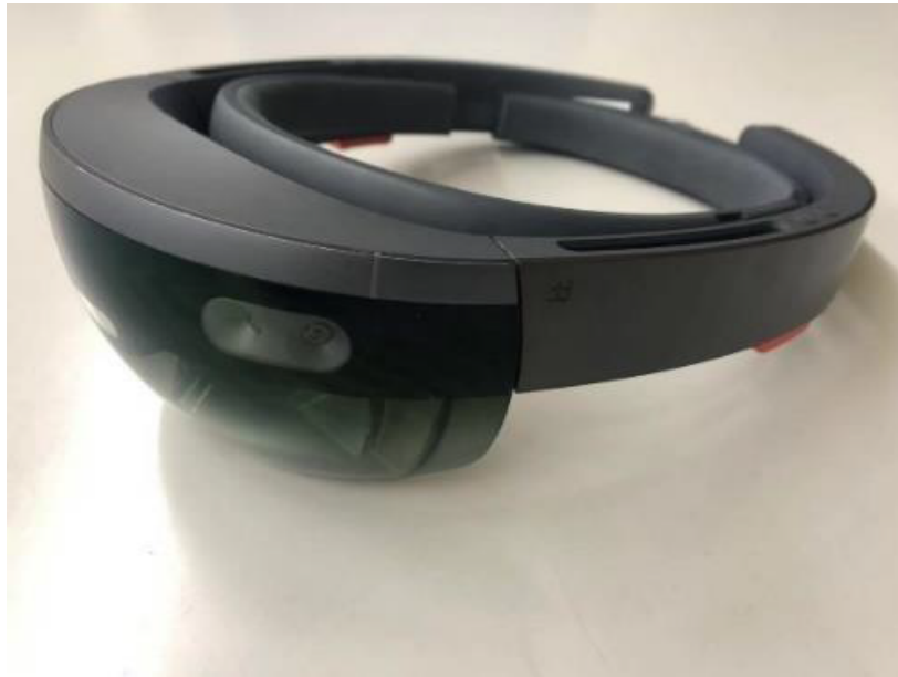
Fig. 5.1 See-through type head-mounted display
