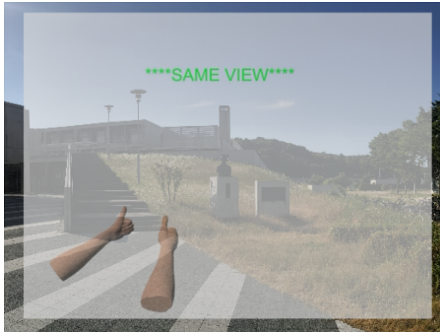
Figure 3.9 Visualization example of the remote user's field of vision. The local user's hands present on the left side, superimposing on the physical world.
