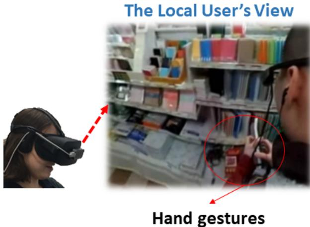
Figure 3. The local user's field of view: the remote user is making gestures
