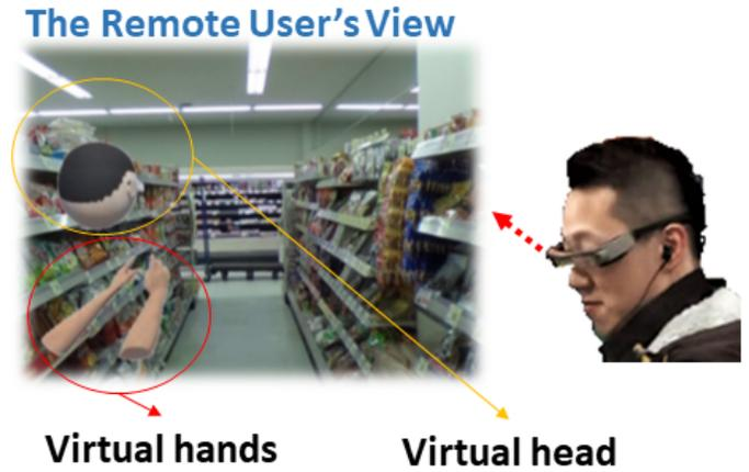
Figure 4. The remote user's field of view: the local user is making gestures. Red circle shows the virtual hands and yellow circle shows the virtual head representing the local user
